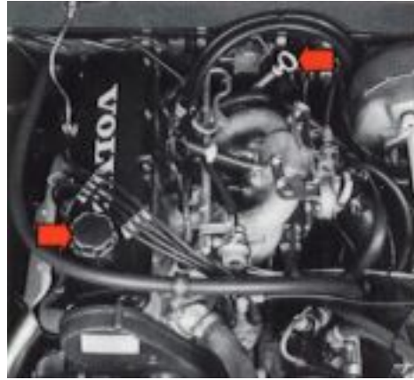
Checking oil level
